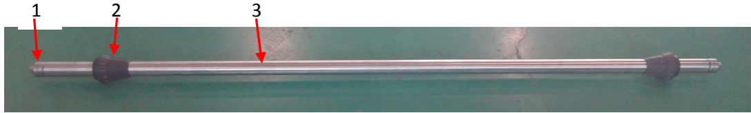
1 Deep groove ball bearings; 2 Chuck 3.stainless steel shaft
